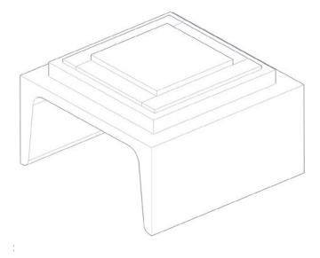
Weld the base plate in the right place following the engineering drawings and using discontinuous welding, trying to minimize the thermal supply due to do not unstuck the PTFE plate. When welding and painting the base plate, you must protect the PTFE plate preventing against spatters.
