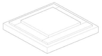
There are two types of PTFE sliding plates. Here is represented the Option 1. In the Option 2 the base plate is drilled due to be fixed on site.
