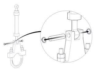
Remove the lower pin and the washers.
