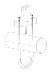
Place the clamp on the pipe. Be careful adjusting the divider, it must lean steady on the pipe.
