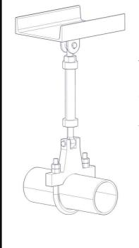
There are different types of sway struts (options 1, 1-A, 2, and 3) depending on different kind of accessories. This guide explains the assembly of a standard sway strut. If the pipe size is not large, the sway strut will be sent pre-assembled. Follow the next steps in order to dismantle the set.
