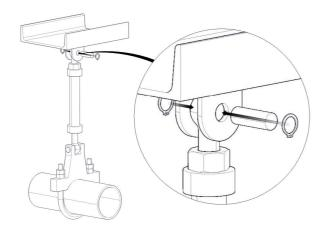
Once the holes are concentric, insert the upper pin and washers.
