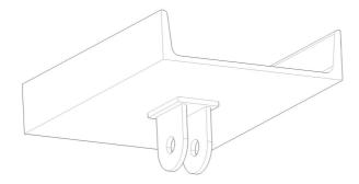
Weld the beam attachment in the right place following the engineering drawings.
