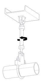
And adjust the length using the extension tube.
