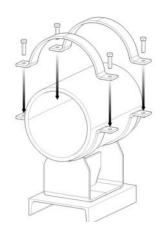
Assemble the clamps and insert the bolts.
