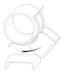
You must place the base clamp under the pipe.
