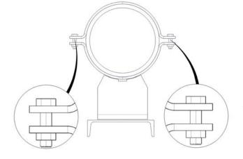
Make sure that the tightening on both sides of the clamps is the same.
